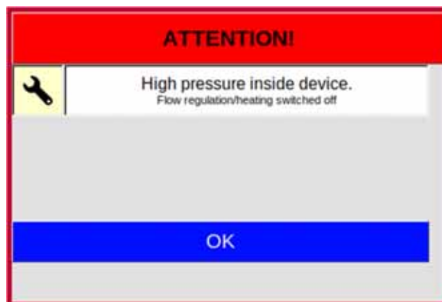
Figure 17: Operating Interface - High Pressure Alarm Box
